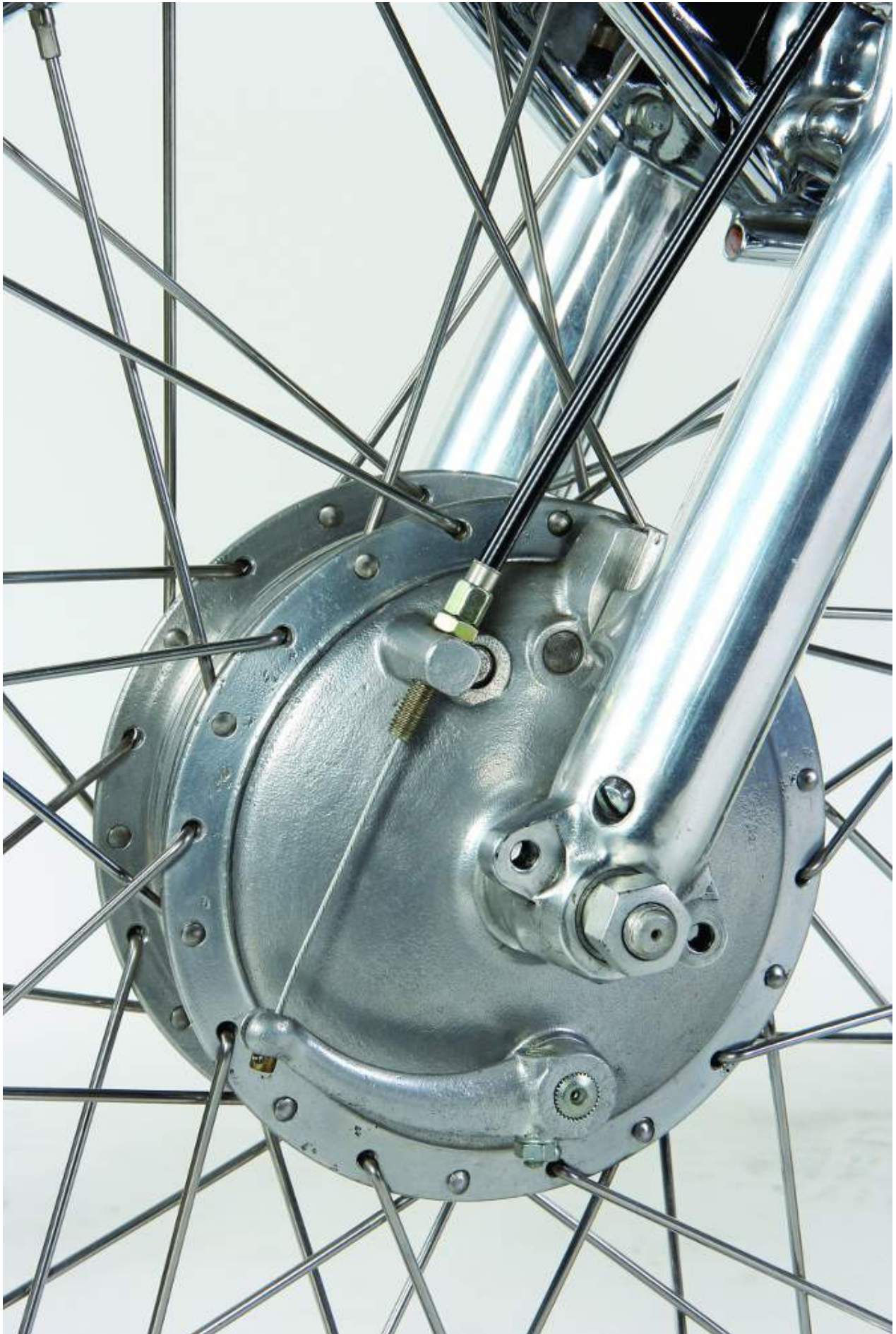
This Monark drum brake was inadequate for stopping a 280 pound race bike,
