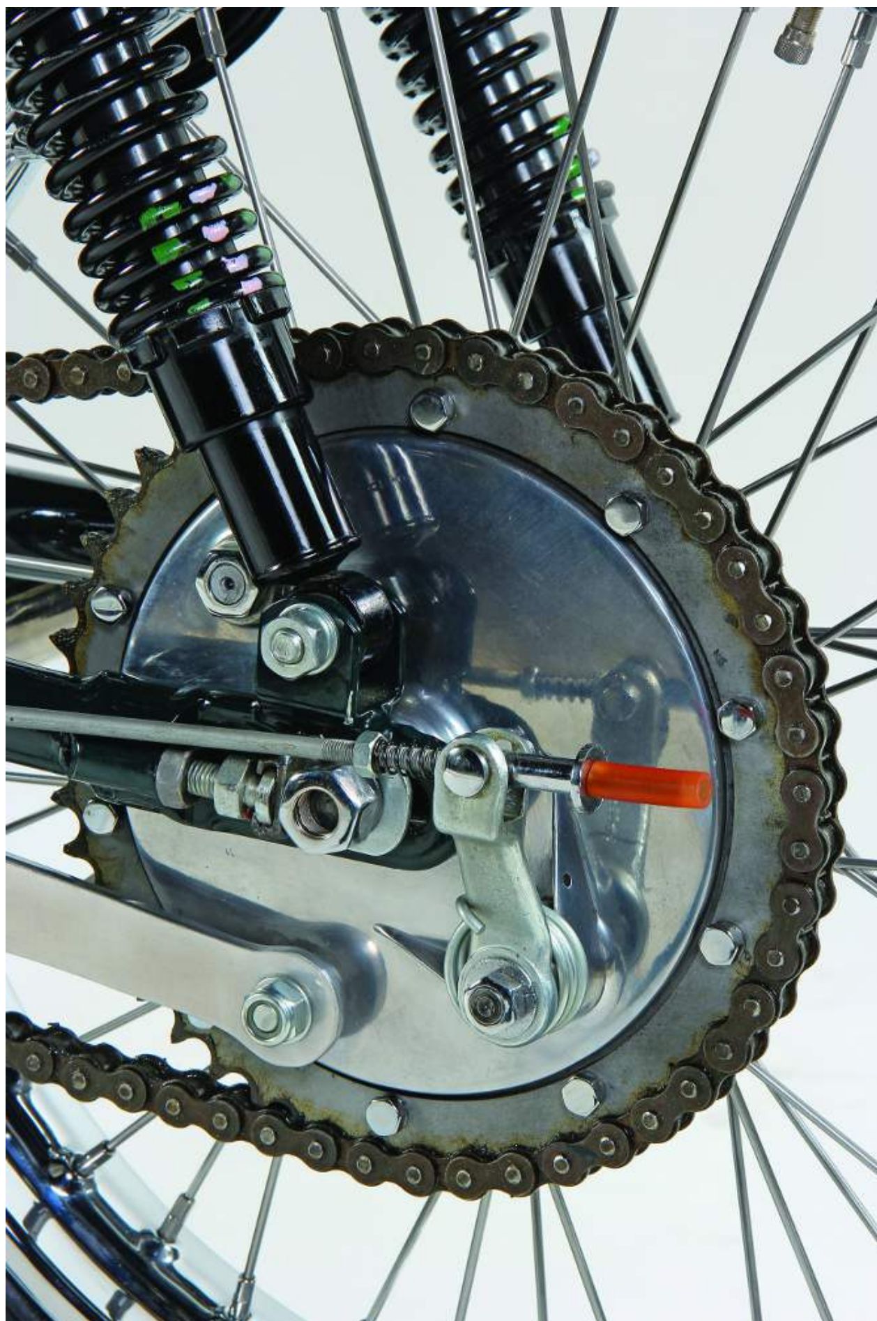
The care taken in building the Lito is evident in the detail of the chain adjuster,
